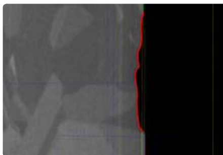
Edge fault on solar cell wafer
