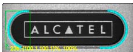
Mobile telephone print located by TemplateFinder3 and PolygonMatch™ with sub-pixel accuracy.
