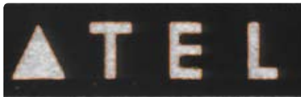
PolygonEdgeFaults2 verifies the edge of the print. The model are translated, rotated and scaled using PolygonMatch technology before edge verification.
